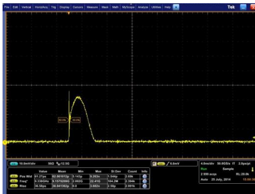
Figure 18 : Example of a 3 nanosecond short pulse (left) driven by Aerodiode CCS pulsed laser diode driver (right). The ~100ps gain switch pulse is observed at the early part of the pulse
